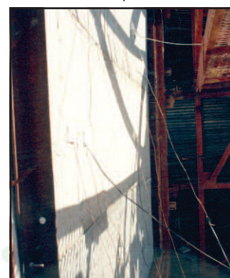
Slight inwards dishing of the panels after 3 hours.
