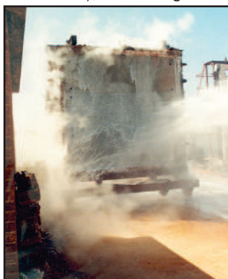
Hose stream application after one minute.
