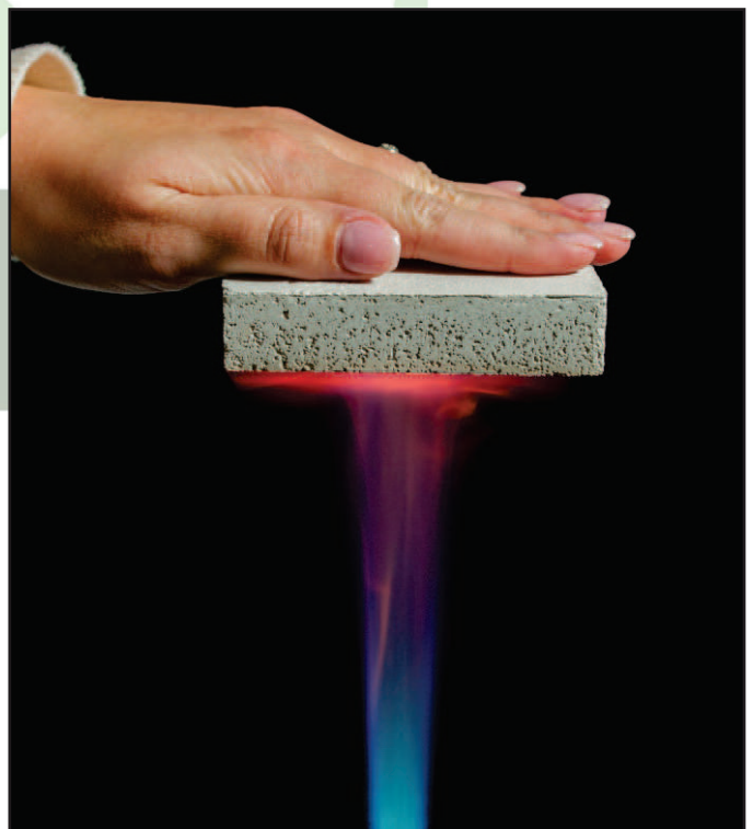
Tudo perlite Concrete is Fireproof and has a low Thermal Conductivity Typical k=0.13 \text{ W/m}^\circ\text{C}
