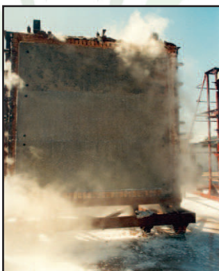
Condition of panels after application of hose steam.
