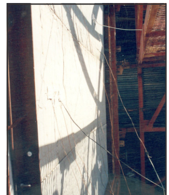
Slight inwards dishing of the panels after 3 hours.
